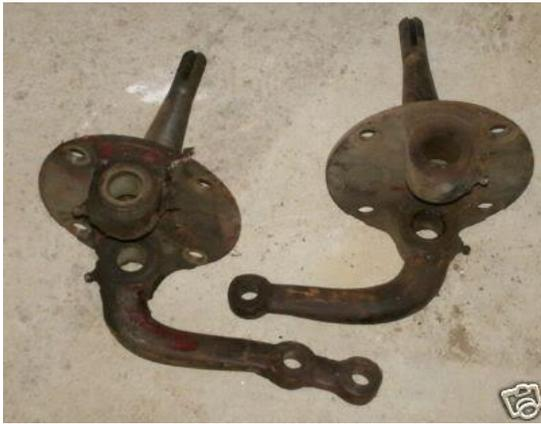
1930's / 40's type Ford Kingpin with forged in steering arm.
