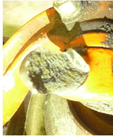
Above - Stub axle showing fatigue crack LH side, which has been present for many years, then recent impact broke it 3/4 through leaving only small section intact which later totally separated. Steering arm , lower section is old partial crack, centre part recent damage, top part held until failing on the day and causing loss of steering.
